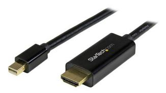
This 6-foot Mini DisplayPort to HDMI adapter cable offers a single-cable connection from your mDP equipped Microsoft Surface Pro, MacBook or Ultrabook laptop to an HDMI display or projector. The passive adapter supports video resolutions up to Ultra HD 4K and is Thunderbolt compatible when connected directly to a supporting DisplayPort over Thunderbolt I/O port.
